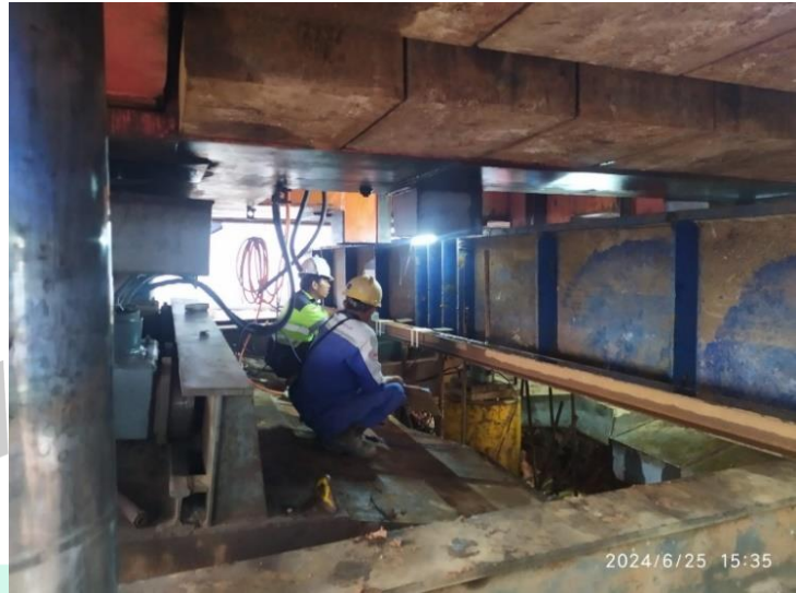
Gambar 3. 32 Loading Test Tekan
