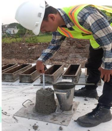
**Gambar 2. 8** *Slump Test*
