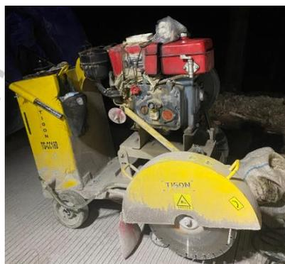
**Gambar 3. 16 Concrete Cutter**
