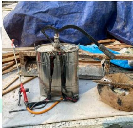
**Gambar 3. 15 Curing Sprayer**
