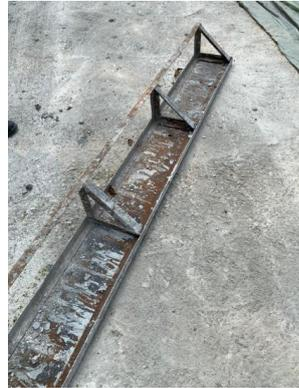
**Gambar 3. 19** *Bekisting Hollow*
