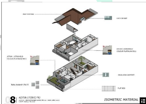
Gambar 3.6. Diagram Isometric Material PKJ House Praktikan (2024)
