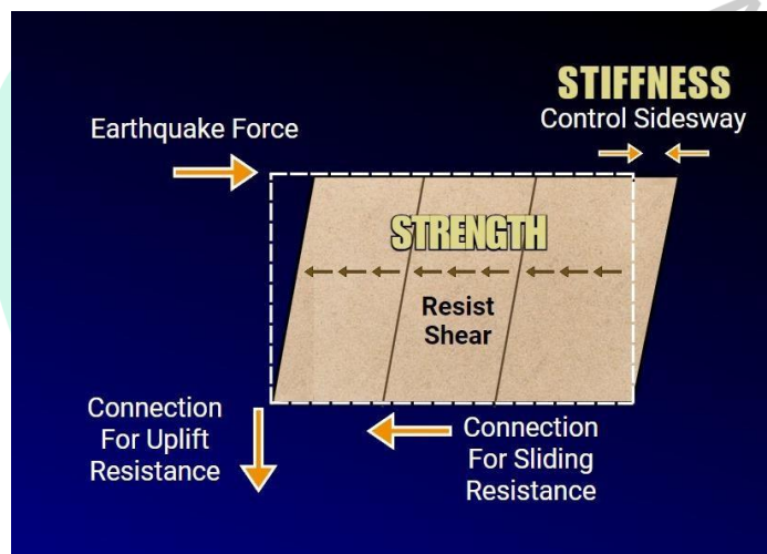
Gambar 3. 35 Diagram Gaya Geser (Sumber: Jurnal Earthquake Engineering and Structural Dynamics Andrew Whittaker dan Thomas C. Hutchinson).
