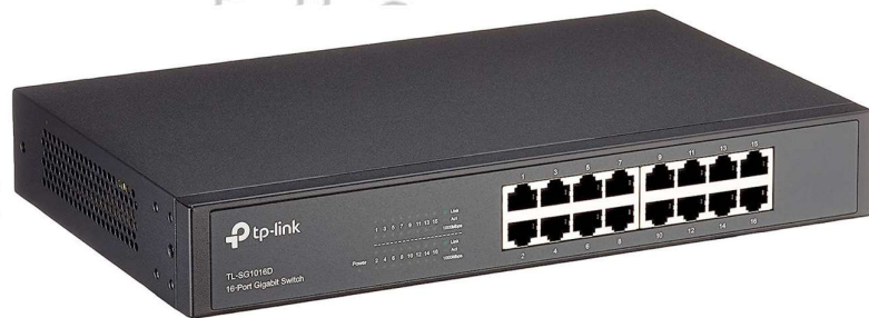
Gambar 3.13 Switch TPLINK TL-SG1016D
