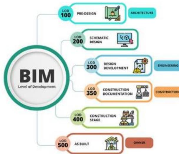
**Gambar 2. 2** BIM Level of Development (LOD)
