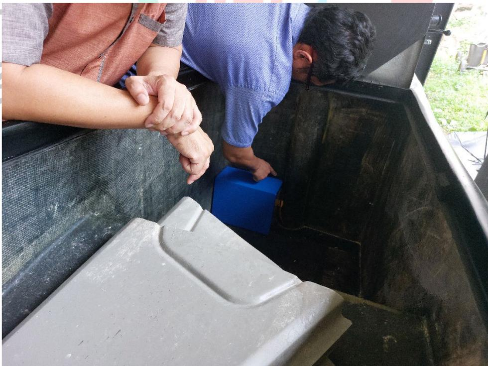
Gambar 3. 34 Fitting Fixed Baterai (2)
