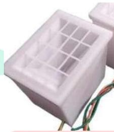
Gambar 2.4 Sensor Tipping Bucket
