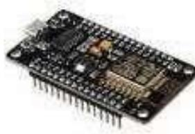
Gambar 2.1 NodeMCU ESP8266
