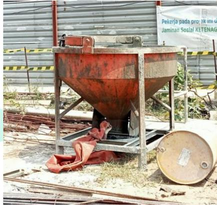
**Gambar 3. 13 Concrete Bucket**
