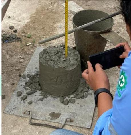
**Gambar 3. 21 Alat Slump Test**
