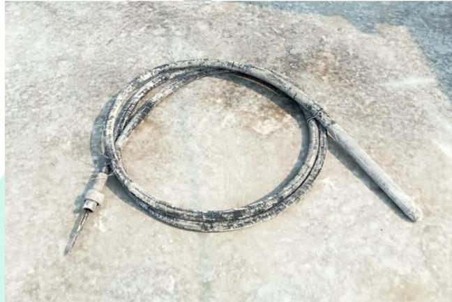
**Gambar 3. 23 Vibrator Internal**
