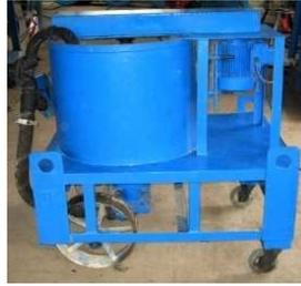
**Gambar 3.18 Grout Pump**
