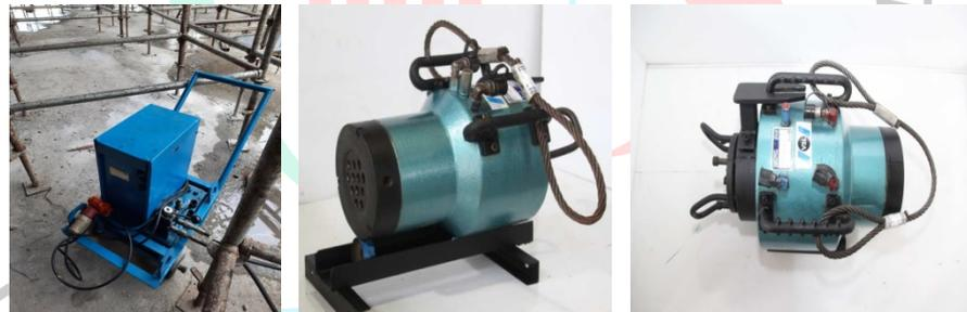
**Gambar 3.17 *Gauge logic*, dan *stressing jack***
