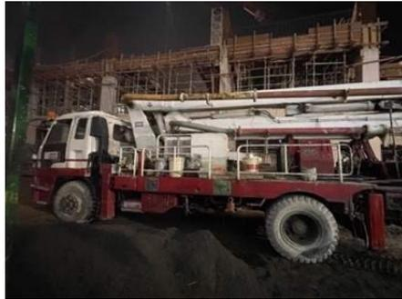
Gambar 3.10 Concrete Pump
