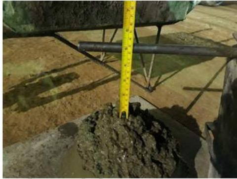
Gambar 3.50 Hasil *Slump Test*
