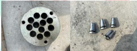
**Gambar 3.32 Wedges Plates dan Wedges**
