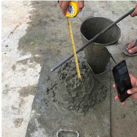
Gambar 3.15 Cek Slump Test Kolom
