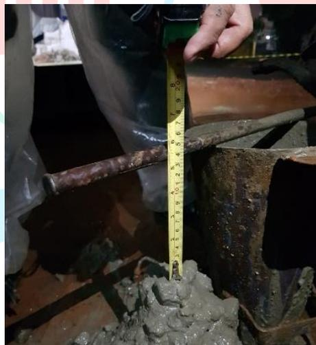
Gambar 3. 26 *Slump Test*
