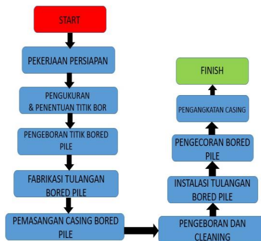
Gambar 3. 2 Flow Chart Pekerjaan Bored Pile
