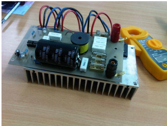
Figure 9. Physical appearance of the module. The Vout terminals have not been soldered at the time the photograph taken. Underneath the PCB is the heatsink on which the transistors are firmly placed.
