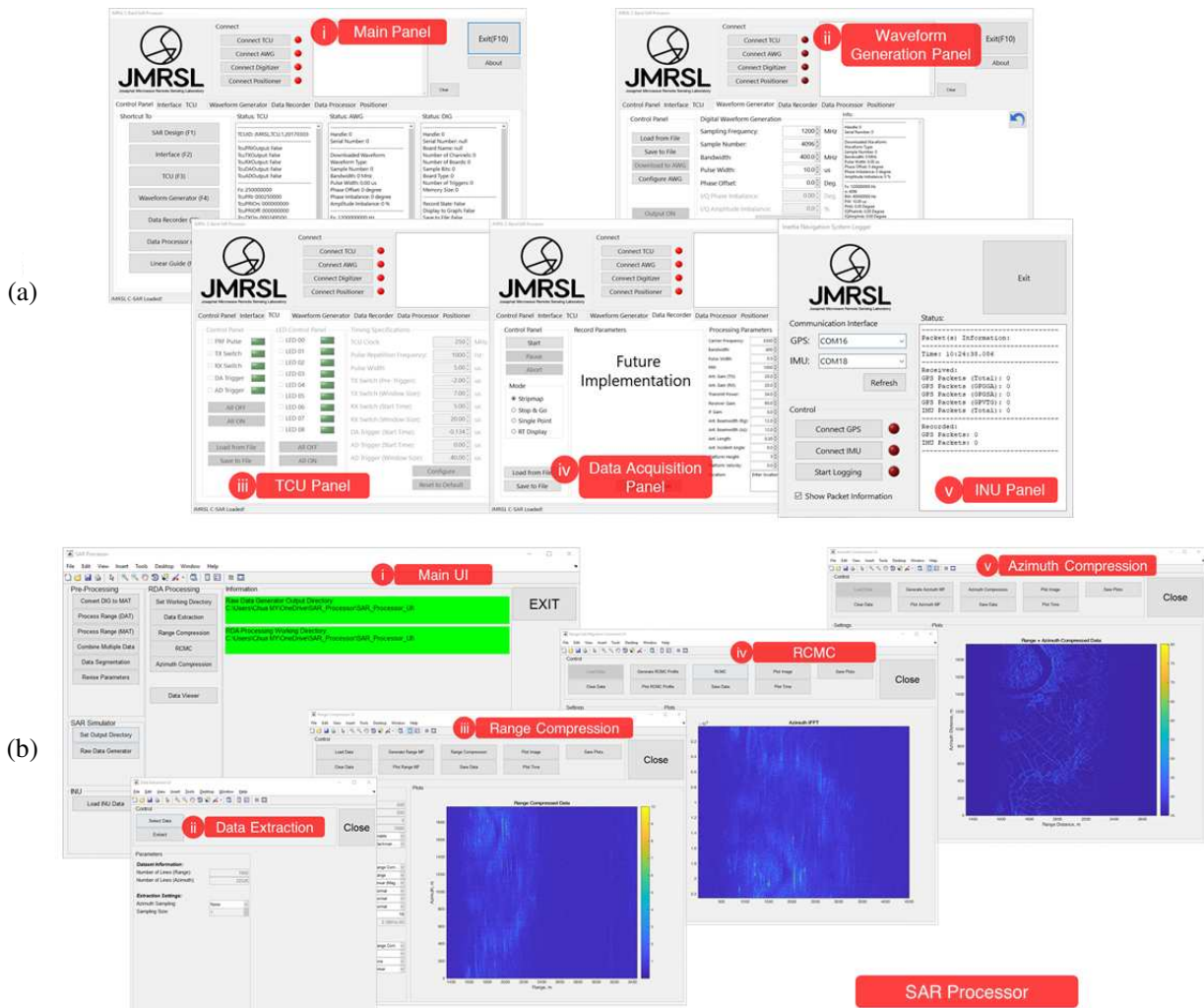
Figure 3. Hinotori-C CP-SAR Software GUI: (a) Control. (b) Image formation.
