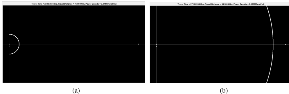
Figure 5: This figure shows states of the simulation at two different time steps of the first leg: (a) is at an early time step, that is, a while after the wave departed from the Tx antenna, (b) is at a late time step, that is, when the wave is approaching the corner reflector.
