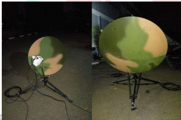
Gambar 2.9. VSAT Disaster Quick Rapid Communication
