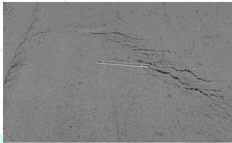
Gambar 2.7 Retak Slip (*Slippage Cracking*) (ASTM D 6433 – 07)
