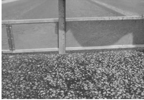
Gambar 2.8 Alur (*Rutting*) (ASTM D 6433 – 07)
