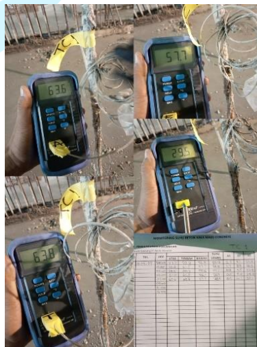
Gambar 3.55 Hasil monitoring suhu beton mass concrete raft foundation (Dokumentasi Pribadi, 2022)
