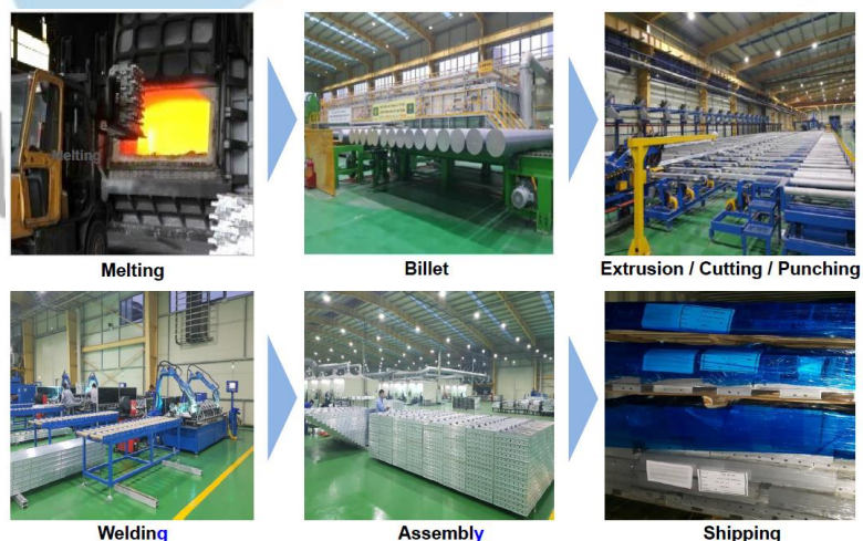
Gambar 3.45 Proses Fabrikasi Aluminium Formwork
