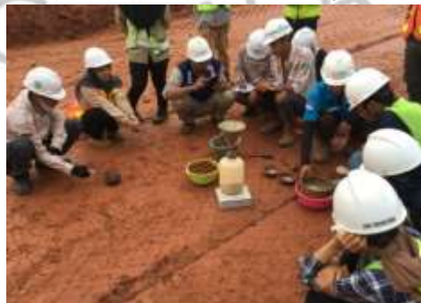
Gambar 3.33 Proses Uji Sandcone
