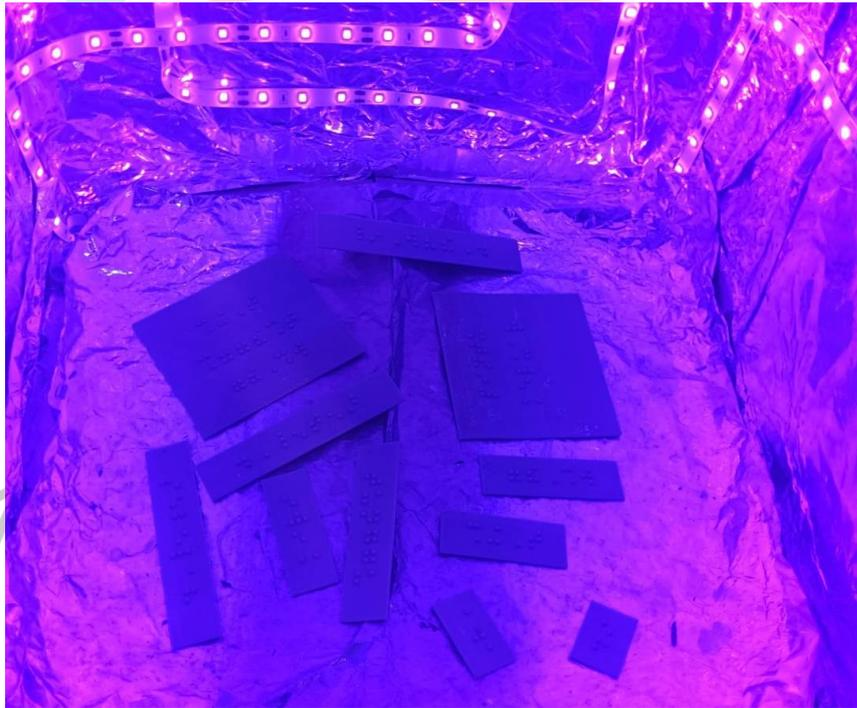
*Gambar 4.27 Proses sinar UV pengeringan model braille plate*
