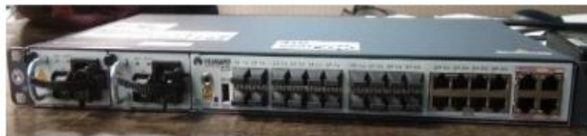
Gambar 3. 7 ATN Switch 910 C-B
