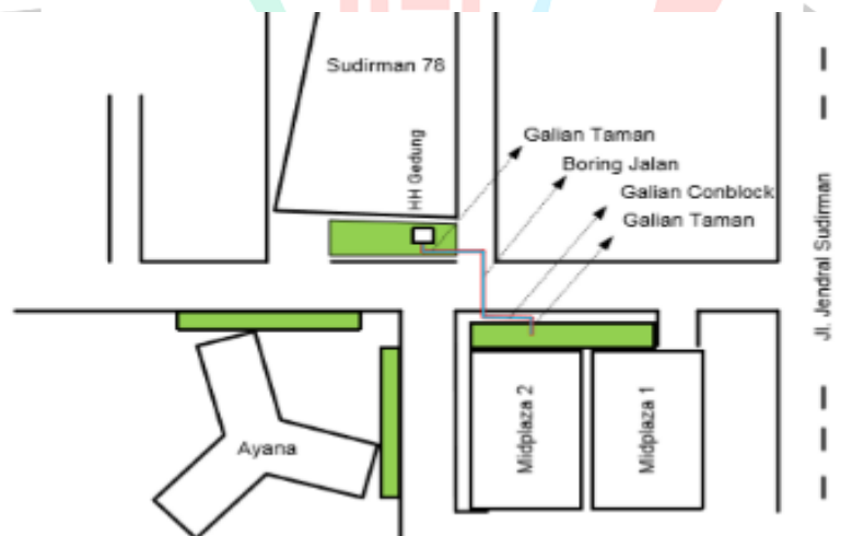
Gambar 3. 19 Diagram Jalur Kabel Backbone Midplaza - Sudirman 78
