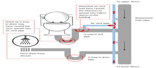
Figure 3: Representation of building plumbing system. Viral particles that are released into drainage could get trapped in the piping system. If the viral particles become aerosolised, the piping system could be the mode of transmission for virus spread within the closed building area.
