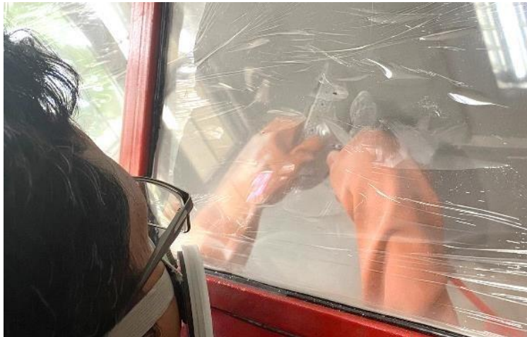
Figure 5. Engraving using sandblasting
