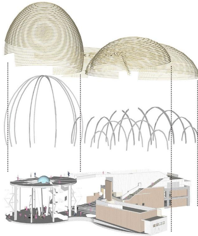
Gambar 2. 4 Struktur Atap Touyan Sewage Treatment Sumber: Archdaily, 2017
