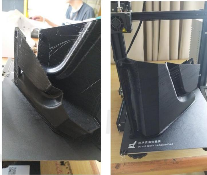
**Gambar 3. 19** Proses 3D Print Body Samping
