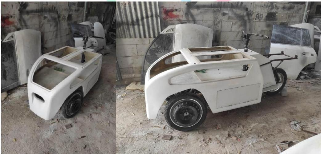
**Gambar 3. 31** Cargobike Fitting Chassis
