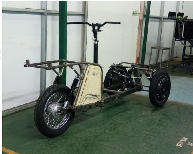
**Gambar 3. 26** Rangka Set Cargo Bike
