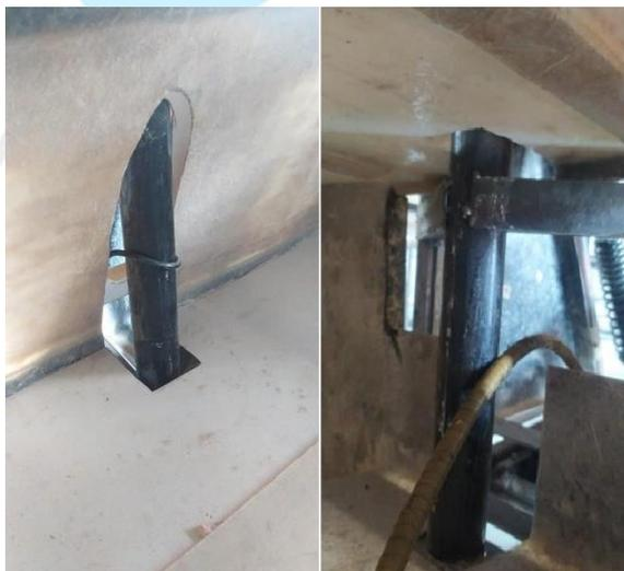
**Gambar 3. 24** Fitting Steering Dengan Crago Box
