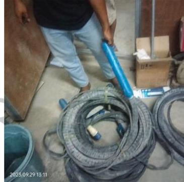
Gambar 3. 20 Vibrator Concrete
