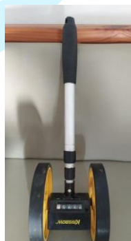
Gambar 3. 6 Meteran Jalan/ Measuring Wheel
