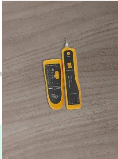
Gambar 3.4 Wire Tracker Cable Tester
