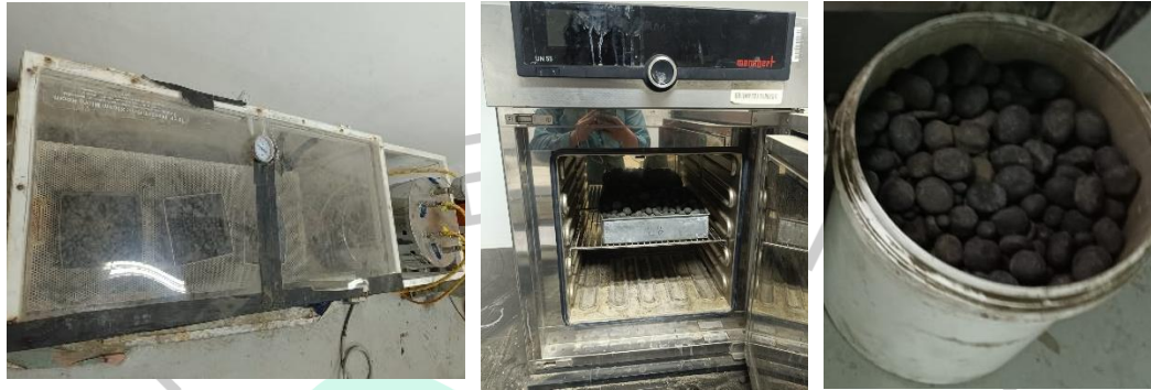
Gambar 4. 8 Proses Curing Steam, Curing Oven, dan Curing Suhu Ruangan
