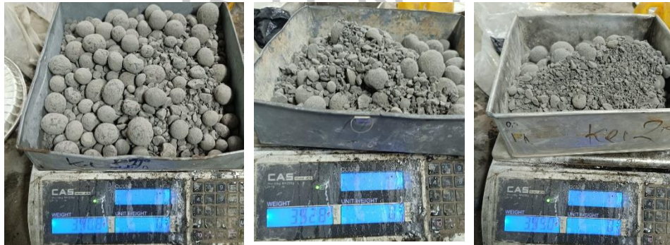
Gambar 4. 14 Hasil Pengujian Los Angeles variable 0%
