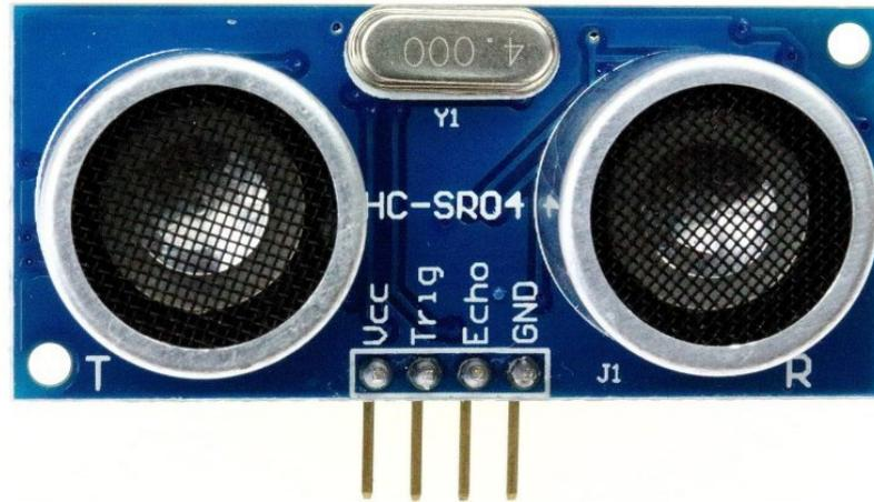
Gambar 2. 8 Sensor ultrasonik distance
