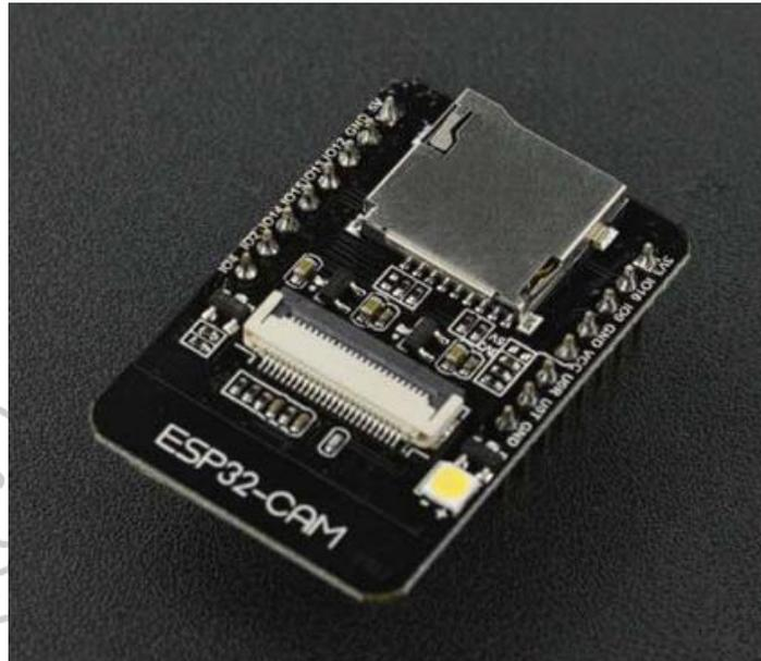
**Gambar 2.4 ESP32-CAM**
