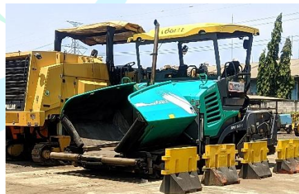
Gambar 3. 30 Asphalt Finisher (Source: Dokumen Pribadi)
