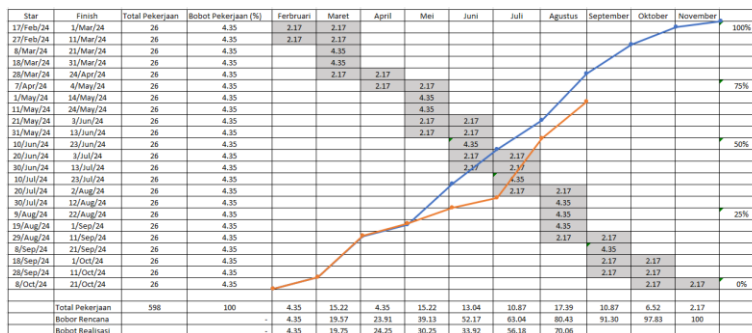
Gambar 3.7. Kurva S Pekerjaan Acian Dinding Sumber: Mapping Apartemen Emerald Bintaro Tower C, 2024
